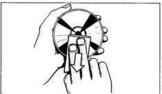
The mechanism of the CD player is fitted with self-lubricating bearings and therefore must not be oiled or greased. English
